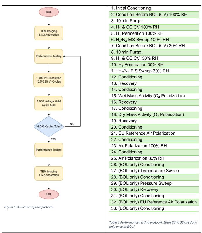
However, before the AST cycles are carried out, a wide range of model parameters can already be extracted from data on materials properties, structure and composition (see D2.2 report). To capture the particle radius distribution (PRD) of the Pt particles within the catalyst layer, TEM imaging is applied. With
